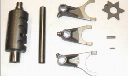
Gearshift drum inspection
