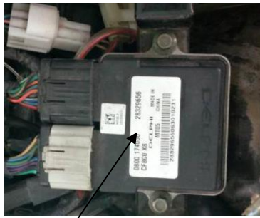
Electronic control unit( ECU)
