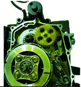
Clean up the seal surface
